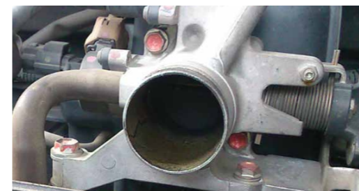
BEFORE (Throttle body condition after 60,000 km)
