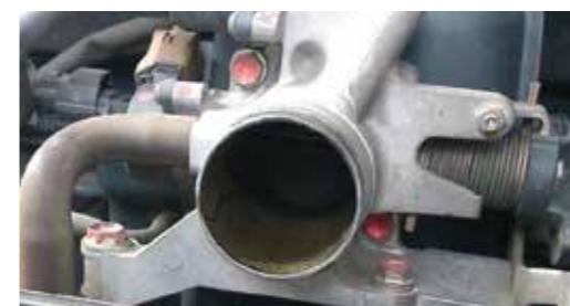
BEFORE (Throttle body condition after 60,000 km)
